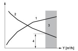
Power output of the heating or cooling registers 1 Differential temperature between supply and return
