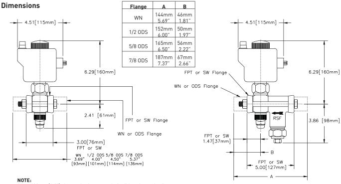
Allow 100mm (4.0") above valve for removal of coil housing and coil. Allow 25mm (1.0") below valve to operate manual opening stem.
