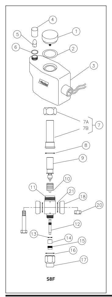
Solenoid Coil is de-energized, allowing #9 Solenoid Plunger to drop and Valve Needle to close the Pilot Port in #10 Piston Plug. Liquid and/or gas leakage through the clearance area around #10 Piston Plug causes a rapid pressure build up in Chamber A which combines with the downward force of the Spring which is part of #9 Solenoid Plunger and the weight of #10 Piston Plug Assembly to force the Main Valve Disc tight against the Seat Bead to stop all flow.
