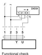
Control with 4...20 mA via external resistor
