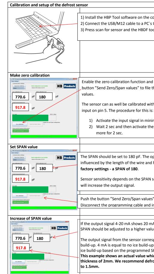
1) Install the HBP Tool software on the computer. 2) Connect the USB/M12 cable to a PC's USB port. 3) Press scan for sensor and the HBDF tool opens up
