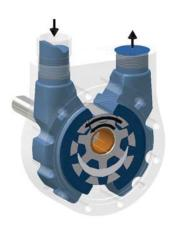
As the pump starts, the teeth come out of mesh, increasing the volume. This creates a partial vacuum, drawing the liquid into the pump through the suction port.
