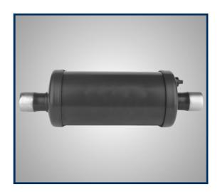
Mufflers have internal baffles designed for minimum pressure drop. These baffles change the velocity of the discharge gasses passing through the muffler. This results in a dampening effect on high frequency sound waves on high speed compressors. Pulsating waves are also muffled in both low speed and high speed compressors.
