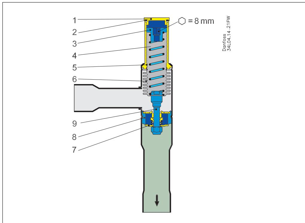
The Crankcase pressure regulator type KVL opens at pressure fall on the outlet side, i.e. when the suction pressure ahead of the compressor drops below the set value.
