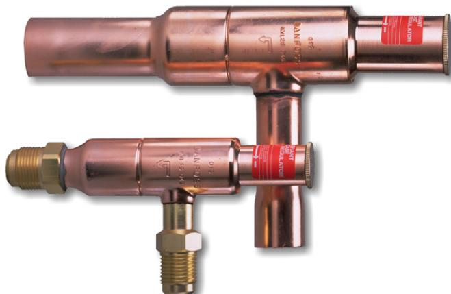
Crankcase pressure regulator type KVL is fitted in the suction line ahead of the compressor. KVL protects the compressor motor against overload during start-up after long standstill periods or after defrost periods (high pressure in evaporator).
