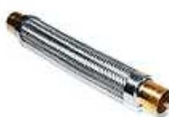
The antivibrators of stainless steel are used in circuits designed with rigid pipelines to obtain a notable decrease of the noises, to absorb and to eliminate the vibrations, and to compensate the expansions produced by the changes of temperature.
