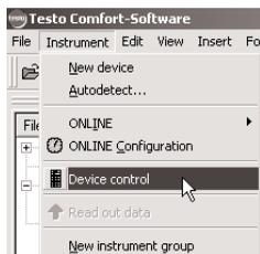
! Programming will result in the loss of any readings that are stored in the device.
